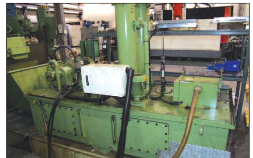
SHIN-IL Gun Drill Hi-pressure coolant system
