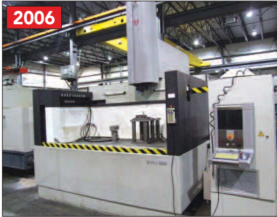
2006 ONA NX8 4-axes CNC Sinker EDM w/orbit
