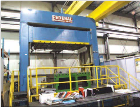
FEDERAL 70 ton Spotting press w/72" x 144" roll-in bolster
