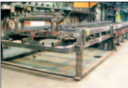
Trailer Transfer Table
