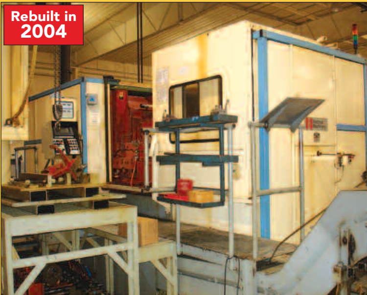
5/8" NATIONAL FORMAX 54-L, 4 DIE 4 BLOW LONG STROKE COLD FORMER
