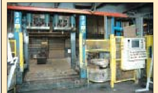
(4) LPM Low Pressure Twin Ram Aluminum Wheel Casting Machines w/Electric Holding Refractory Furnace
