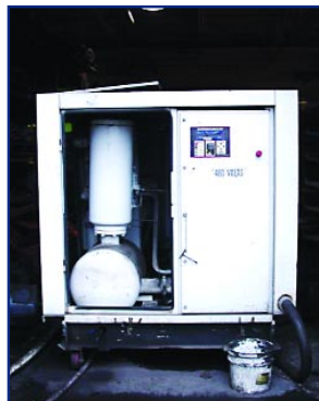
GARDNER DENVER PORTABLE AIR COOLED 150 HP SCREW TYPE AIR COMPRESSOR, MDL. EDM00A
