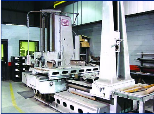
LUCAS HORIZONTAL BORING MILL MDL. 42B-60
