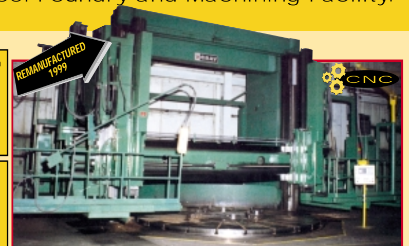
GRAY 16' CNC Vertical Boring Mill (Remanufactured 1999) Over 2 Million Dollars Replacement. (To Be Auctioned June 13th McNally Mfg.)
