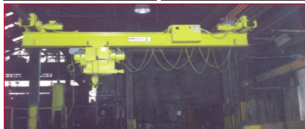
ACE 2 Ton Bridge Crane
